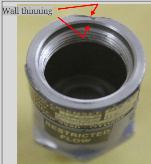
Fig.6: Thinning of the wall of end-fitting due to corrosion
